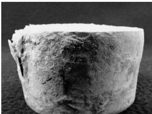
**Fig. 4.** Damage to stone surface of the sample caused by salt crystallization
