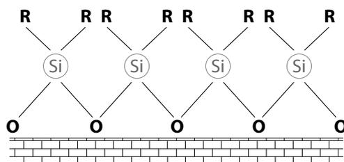
Fig. 6. The principle of organosilicone compounds action
