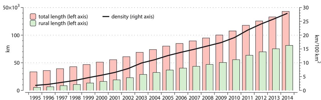
**Fig. 4.** The length and density of sewage systems in Poland in the years 1995–2014
